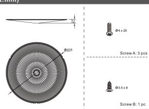
**B. Installation Instruction** 1. 🛠 3. 🛠 2. 🛠 1 1 A x3 Take 3 screws off, keep the other 3. Install the Anti-glare diffuser body to LED high bay with 3 supplied screws. 4. 🛠 6. 🛠 5. 🛠 thr 2.7 Bx1 Put the clips and threaded hole to Push the cover in clockwise direction to make the clips locked tight, fasten the diffuser body and cover with the supplied screw. matching positions.
